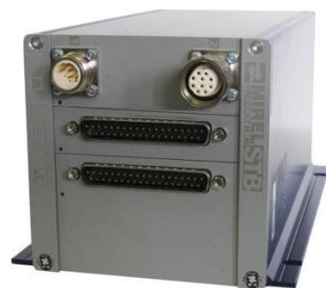
Functional interface MIREL STB is an equipment of the MIREL modular system. Basic function of the MIREL STB is to provide an interface between the train protection MIREL VZ1 central unit and the onboard unit ETCS (function STM). This basic function is realized either by binary or serial interface.
