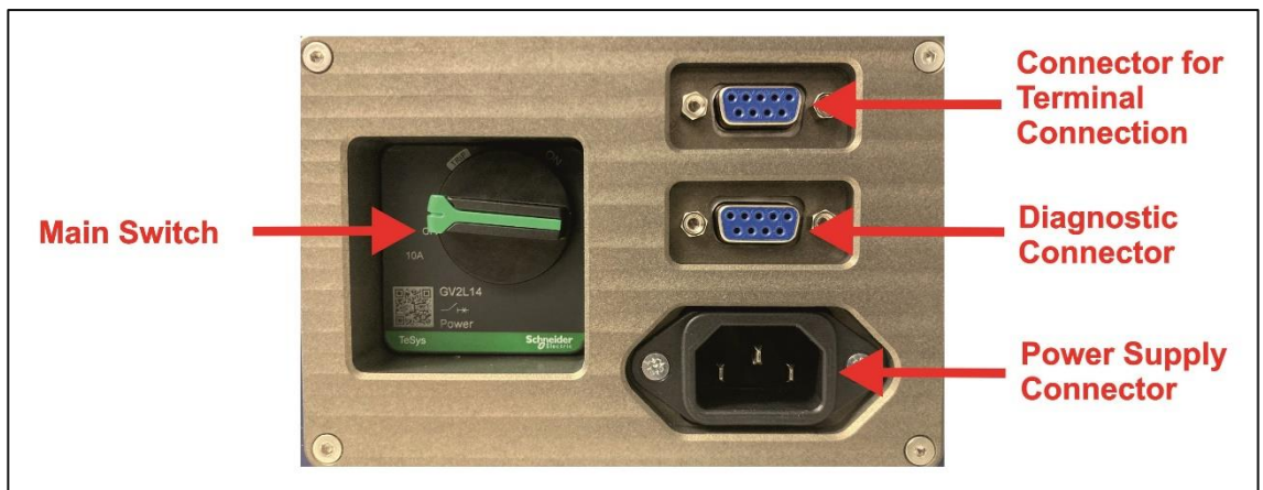
Fig.5b: Description of IRCP.3.A Drive Unit's Main Panel
