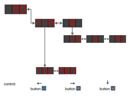
When operating in SHP national mode, it is possible to carry out only switching between national modes. Switching is enabled only on DRV at standstill. Menu shown below serves for switching between national modes during operation in SHP national mode:
