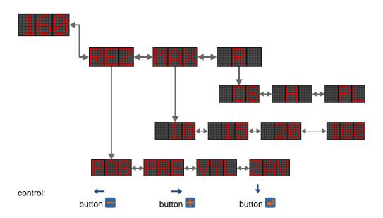
The selection of operating mode when operating in EVM national mode can be carried out at a DRV speed lower than 40 km.h<sup>-1</sup>, without actual speed violation. Switching between national modes is possible only on DRV at standstill. Menu shown below serves for entering of operating parameters during operation in EVM national mode:
