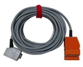
Accessories, connection cable for axle speed sensor simulation serves for connection of VZT.4 control electronics with terminal plate of axle speed sensor on HDV axle. Its length is 8 metres. At side of VZT.4 control electronics (connector No.5) connected by D-sub female connector (left picture side), at the side of HDV terminal plate, the conductor is connected by WAGO – M connector (right picture side).
