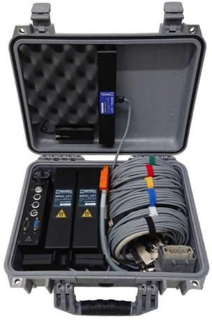
Pictures above show the case design and partition of its internal space. Picture on the right shows an example of storage concerning individual accessories. Accessories cables have been produced from highly flexible and resistant cables intended for frequent stress and have been equipped with colour textile binds in order to achieve easy identification and enabling a better organizing within the case space.
