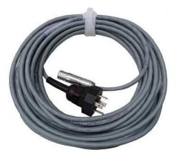
Connection cable accessories for pressure sensor simulation. Cable has a length of 8 meters, at one end terminated by MSCF connector of MiniCon type for connection with VZT.4 electronics (connector No.4), at the other end terminated by industrial circular connector of Type A 3P-PE for connection with connector intended for MIREL ST pressure sensor.
