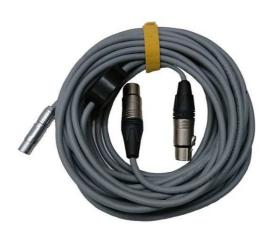
Accessories, connection cable for simulated code transmitters serves for interconnection of KSV transmitters with VZT.4 control electronics. Its length is 10 meters, at one end terminated with MSCM connector of MiniCon type (on left picture), which serves for connection of VZT.4 control electronics(connector No.2). At the other end, the conductor is tees and at both ends it's terminated by connectors of XLR type (in picture centre), which serve for connection of KSV accessories.
