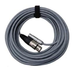
Extension cable of code simulation loop serves for extension of conductor line to KS accessories. Cable has a length of 10 meters, at one end terminated with XLR connector for wiring to KS accessories, at the other end terminated with MiniCon MRM1 connector for wiring to VZT.4 device (connector No.3).
