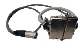
Code simulation loops are positioned on compensating coil of MIREL SN type. Code simulation loops are connected with XLR connector piece (Figure left) to accessories of PPKS extension cable.
