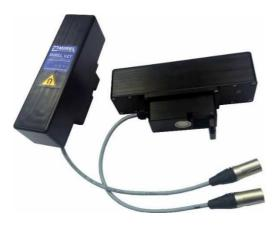
Accessories, simulated code transmitter are situated below the code sensor of MIREL SN type directly on rail. Correct positioning on rail is supported by swivel stop on bottom side. Position is fixed by a permanent magnet in the KSV leg. Placing happens always pairwise and below pair of sensors. PKSV accessories serve for their wiring to control electronics. Standard set comprises two KSV transmitters.
