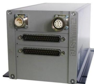
Functional interface MIREL STB is an equipment of the MIREL modular system. Basic function of the MIREL STB is to provide an interface between the train protection MIREL VZ1 central unit and the onboard unit ETCS (function STM). This basic function is realized either by binary or serial interface.
